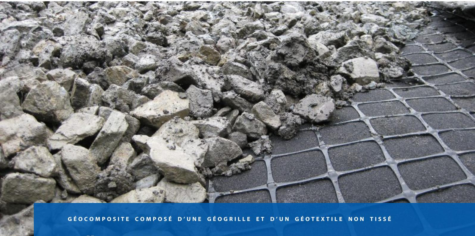
GÉOCOMPOSITE COMPOSÉ D'UNE GÉOGRILLE ET D'UN GÉOTEXTILE NON TISSÉ
